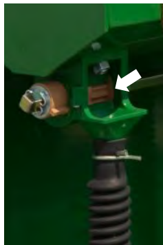
Conventional drill with rotating gear that "spills" seed into the drop tube
