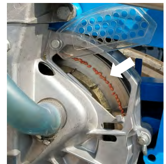
Precision planter with vacuum that picks up individual seeds and drops one seed at a time down the drop tube
