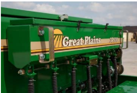
Conventional drill with rotating gear that "spills" seed into the drop tube
